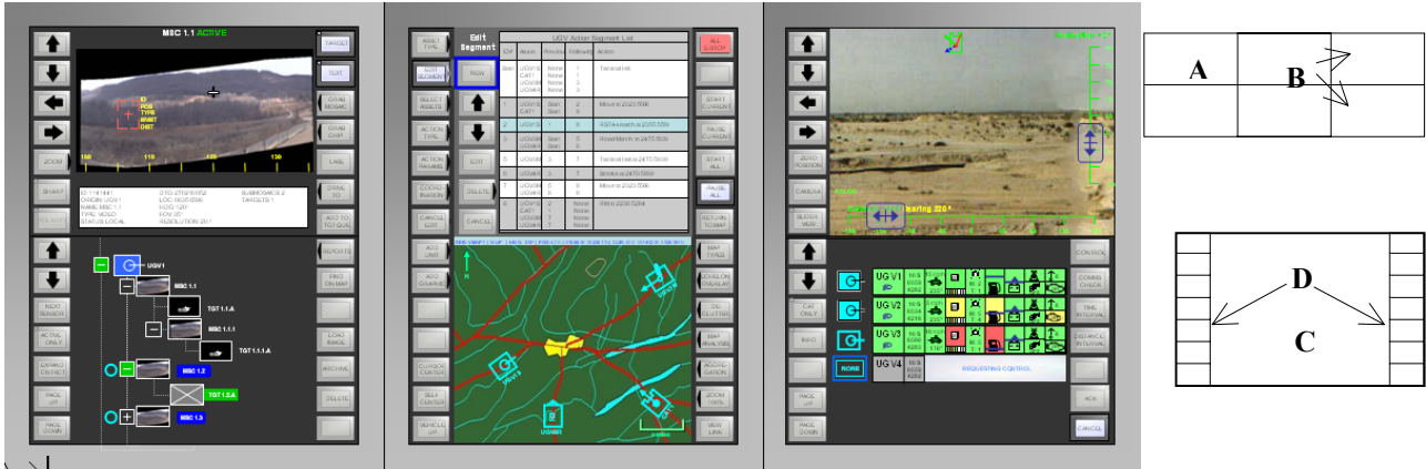
Figure 1. Layout of displays for robotic control using the VTI control station A control station comprises six displays (A). Each 20 inch monitor screen (B) comprises two half-screen displays or one full screen display. Each display has a viewing/interaction area (C) and one or two fixed columns of seven 1" x 1.5" buttons (D). The displays shown are the RSTA viewer /browser (left screen), mission planning (top center), mapping (bottom center), situation awareness camera (top right), and asset control (bottom right). The control yoke is located under the center screen.
