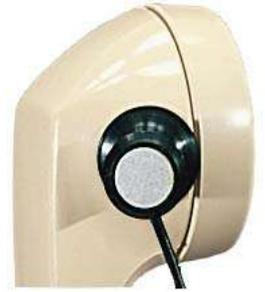
Small magnetic pickup coil that has an attached suction cup, attached to the phone earpiece and picks up both sides of conversation.
